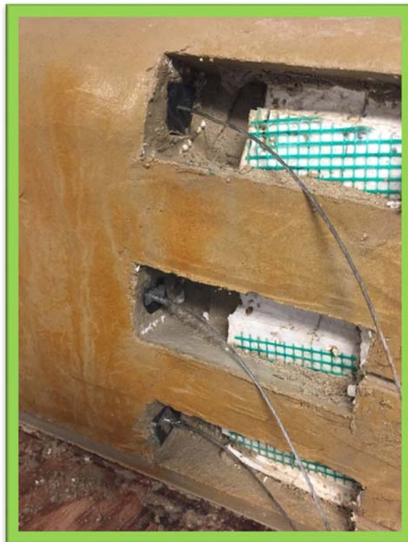
Figure 16: Post Tensioning Canoe 7 Days After Casting
