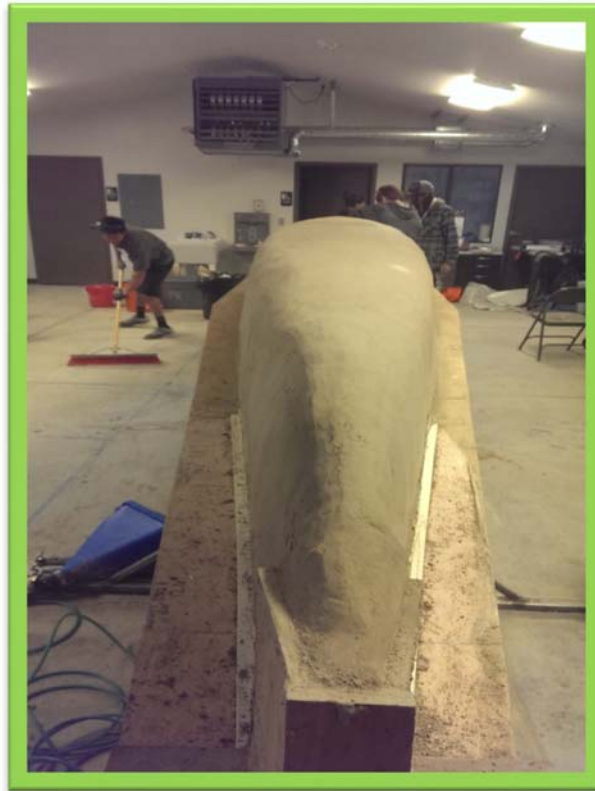
Figure 15: Canoe at Desired 1/2" Thickness
