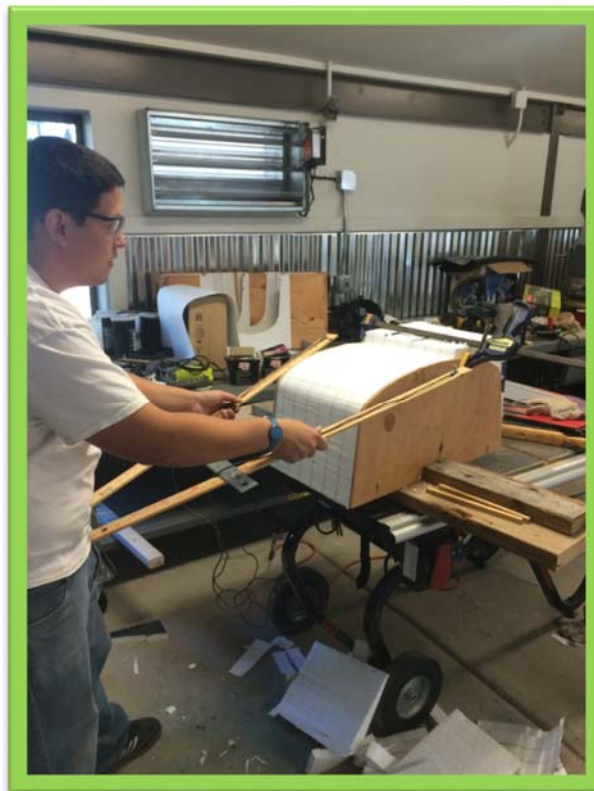
Figure 4: Cutting Foam Cross Sections Using a Hot Wire
