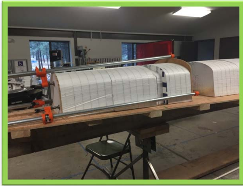
Figure 5: Gluing Sections Together
