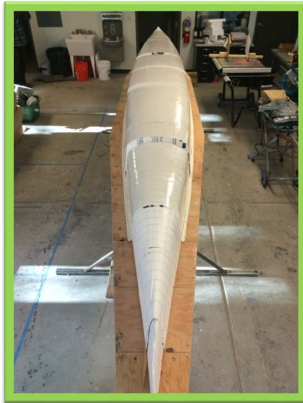
Figure 6: Completed Mold with Shrink Wrap
