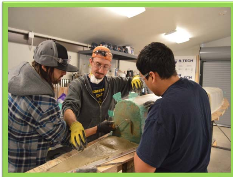
Figure 10: Placement of Flotation for Bulkheads
